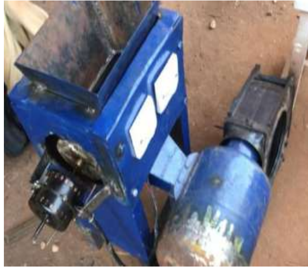
Plate 2: Fabricated Melon Shelling Machine
