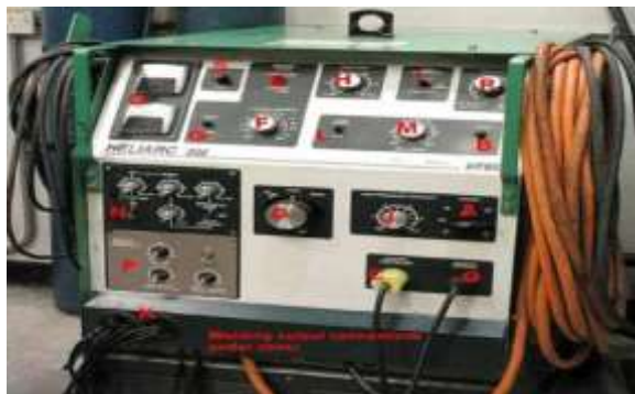
Plate 2: Gas tungsten arc welding machine
