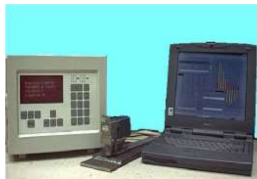
Plate 4: Ultrasonic computerised complex for measuring Residual Stress
