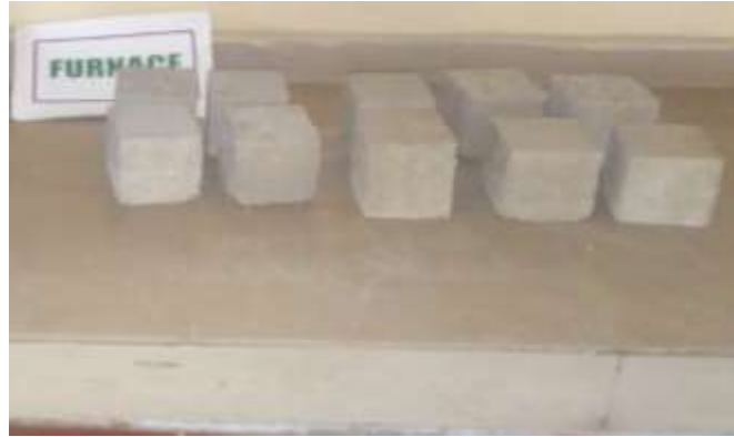
Figure 2 test sample bricks prepared from ovia river clay deposit
