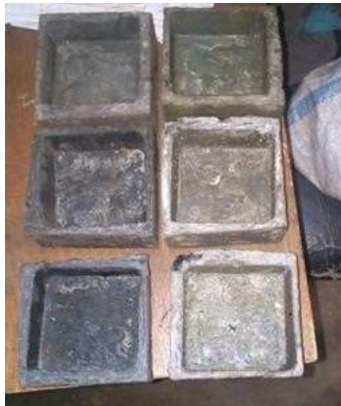
Figure 10 Finished Formed Compression Mould Plastic Products
