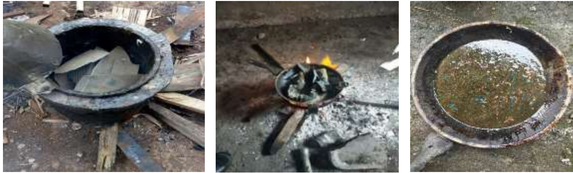
Figure 8. Melting of Feedstock in Wood Fired: (a) Polypropylene melt charge (b) PVC melt charge and (c) Melted PET charge
