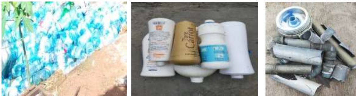
Figure 7. Part of Sorted Plastics: (a) PET Bottles (b) Cream Bottles of HDPE (c) PVC Pipes
